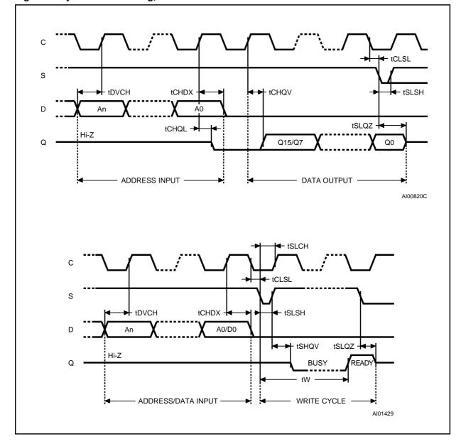
Figure 5. Synchronous Timing, Read or Write
