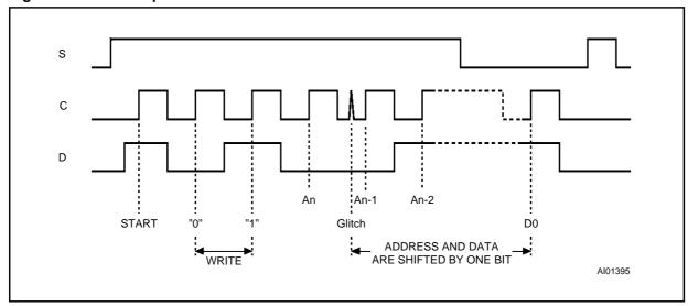
Figure 9. WRITE Sequence with One Clock Glitch
