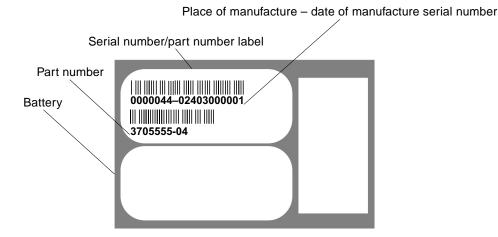
As shown in the previous figure, the serial number/part number label on the battery has two bar codes. Below the upper bar code is a seven-digit Sun-supplied place of manufacture, followed by a dash (-) followed by a four-digit code that indicates the date of manufacture, followed by a six-digit supplier-assigned serial number.
