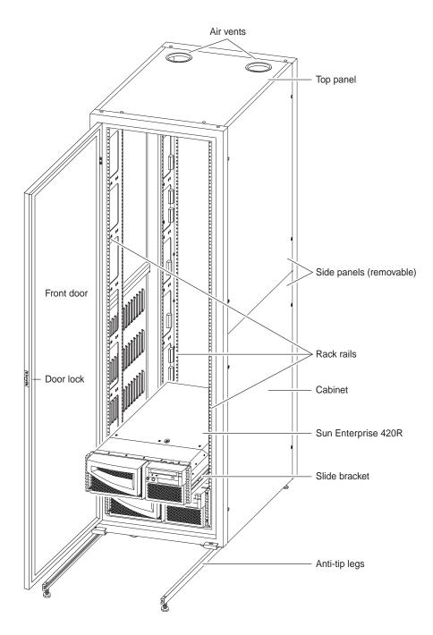
FIGURE 1-1 Systems Mounted in a Cabinet and Rack
