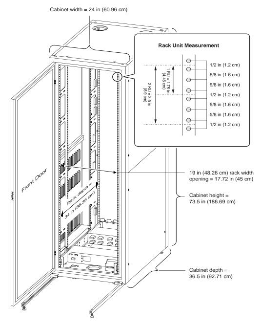
FIGURE 2-2 EIA 310-Compliant Cabinet and Rack
