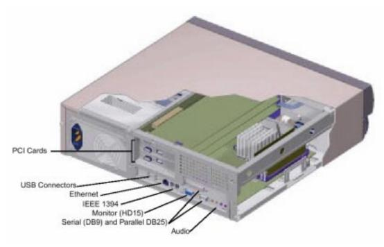
Figure 3. Rear view of Sun Blade 100 workstation, showing connectors
