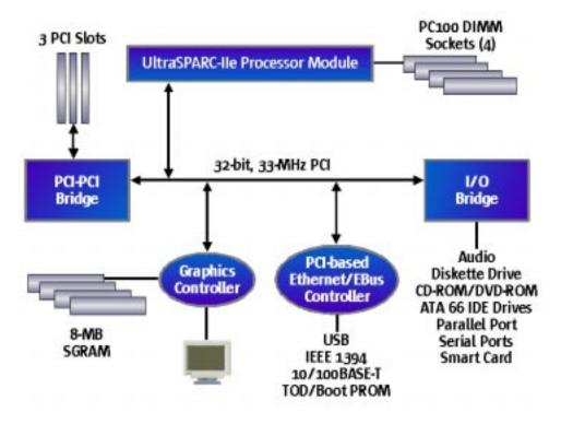
Figure 2. Sun Blade™ 100 workstation system block diagram
